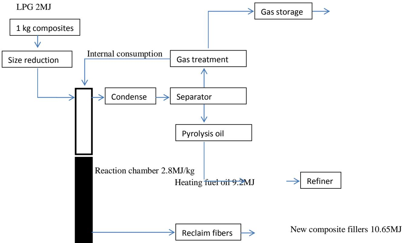
Figure 5: Schematic diagram of pyrolysis for composites and energy credits. Source: Scheir (1998)
