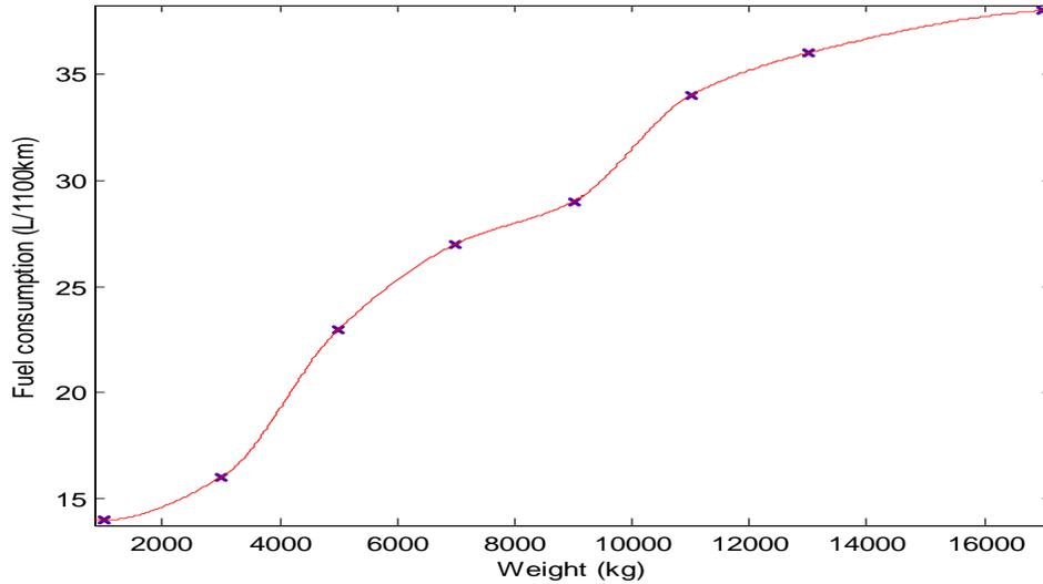
Figure 3i: Fuel efficiency with respect to curb weight for heavy vehicles [47]
