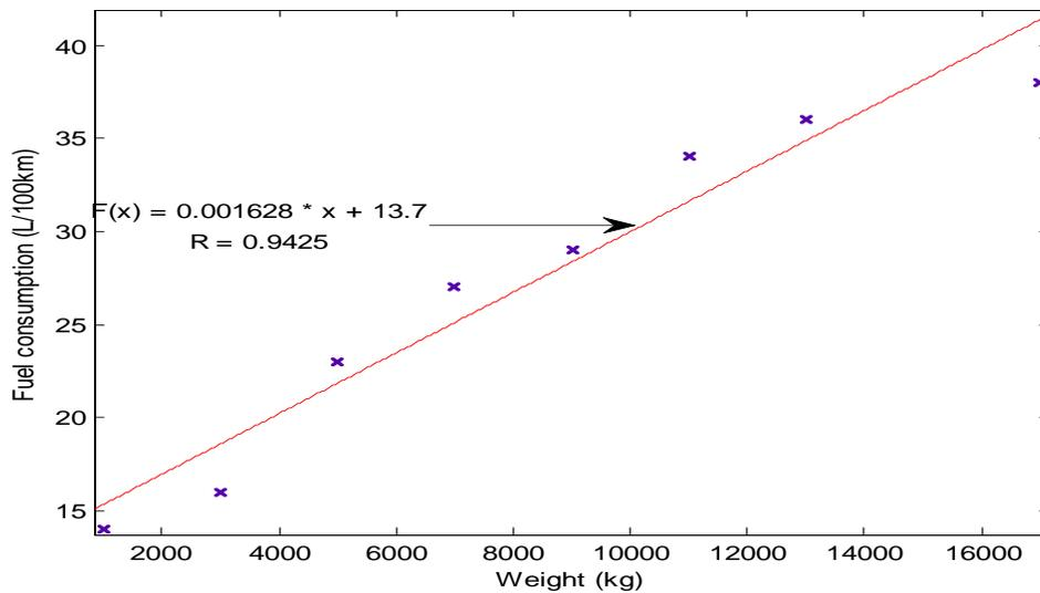
Figure 3ii: Linearized fuel efficiency with respect to curb weight for heavy vehicles [47]
