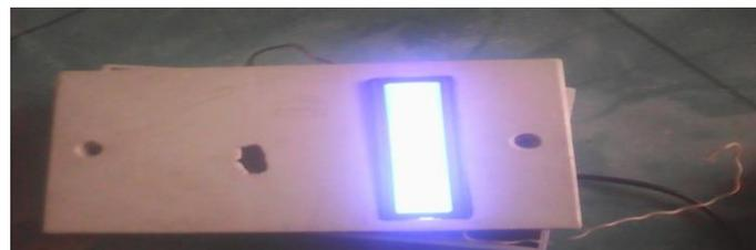
Figure 8: Digital thermometer taking reading from the environment
