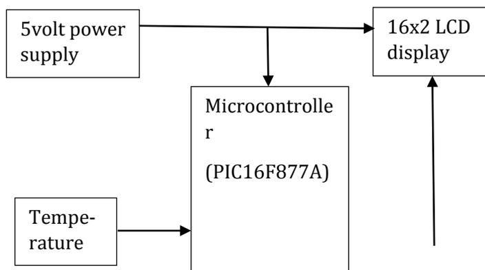
Figure 1: Block Diagram of Digital Temperature Meter (Srireddy, 2009)
