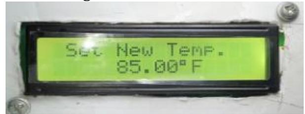
Figure 4. 7: Temperature Set Display
