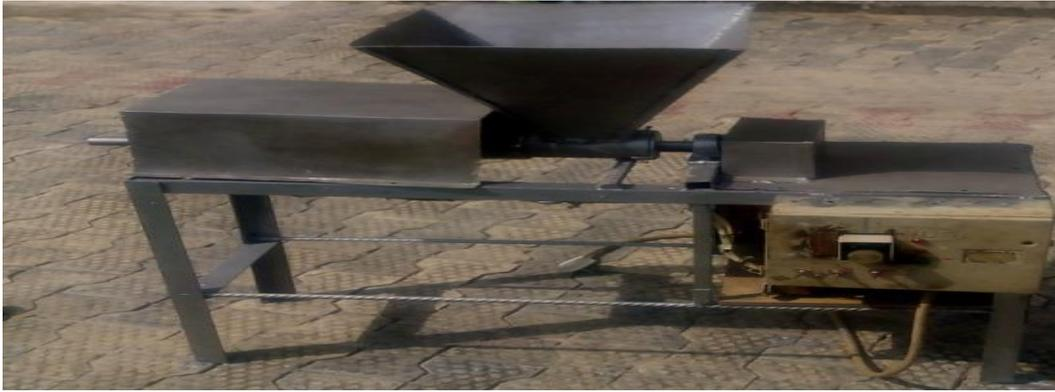
Figure 2: The Designed and fabricated low density pilot Polythene recycling system
