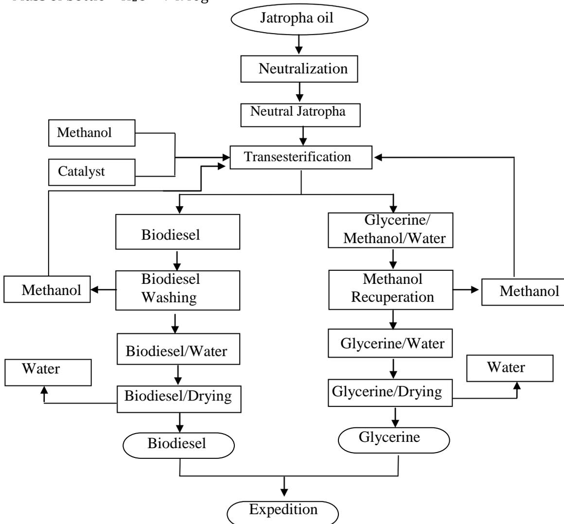
Figure 1: Schematic process diagram of Biodiesel
