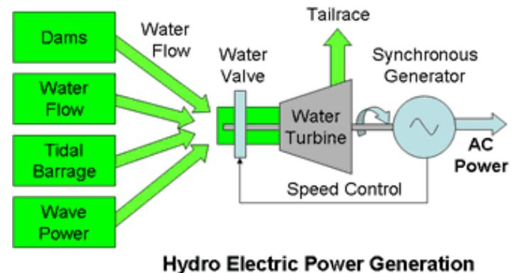
**Water Turbines:** Like steam turbines, water turbines may depend on the impulse of the working fluid on the turbine blades or the reaction between the working fluid and the blades to turn the turbine shaft which in turn drives the generator. Several different families of turbines have been developed to optimize performance for particular water supply conditions.
