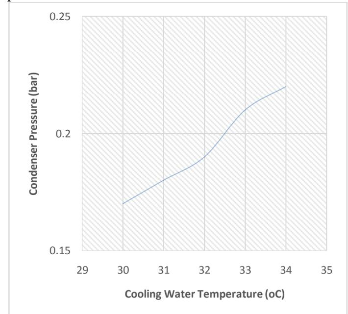
Fig. 2: Variation of Condenser Pressure with Cooling Water Temperature
