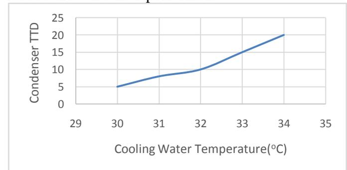
Fig. 4: Variation of Condenser TTD with Cooling Water Temperature
