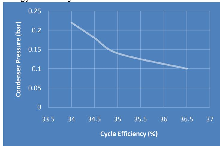
Figure 3. Variation of Cycle Efficiency with Condenser Pressure
