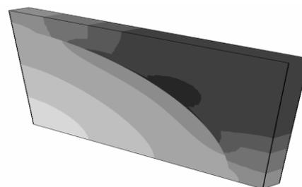
Figure 1: Contour plot of the maximum principal residual stress (N/mm<sup>2</sup>) for  $V_f = 60\%$ .
