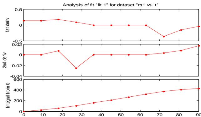
Figure2a: Analysis fit for distribution of the max principal residual stress in resin along fiber/matrix interface ( $V_f= 60\%$ ).
