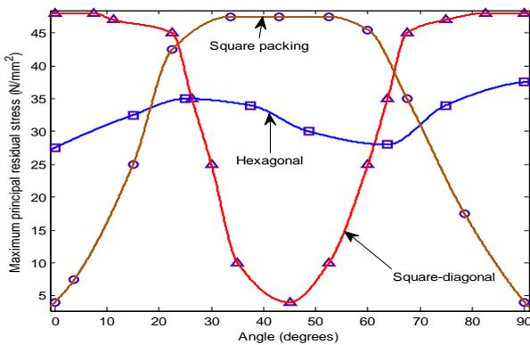
Figure 4: Distribution of the maximum principal residual stress in the resin along the fiber/matrix interface for three different fiber packing (fiber volume fraction  $V_f= 60\%$ ).
