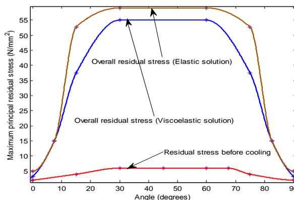
Figure 2: Distribution of the maximum principal residual stress in the resin along the fiber/matrix interface for  $V_f = 60\%$ .
