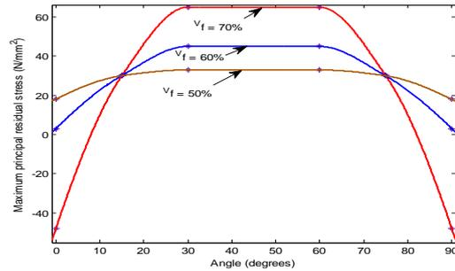
Figure3: Distribution of max principal residual stress in resin along fiber/matrix interface for three different fiber volume fractions.
