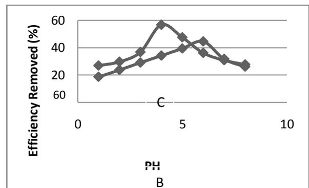
**Figure 3: Effect of pH variation on potassium permanganate removal using corn cob and animal bone derived adsorbent.**
