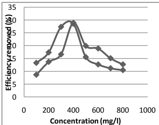
**Figure 1: Effect of different initial dye concentration on dye removal using CC and AB derived adsorbent.**
