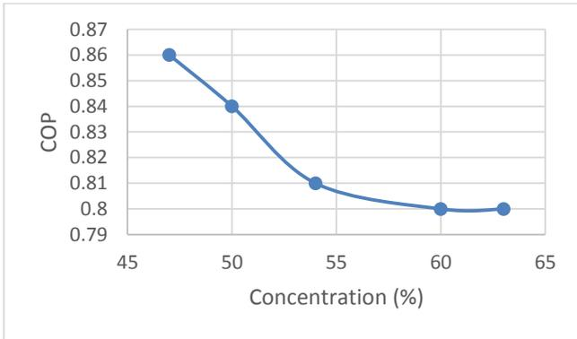
Figure 3: Concentration of LiBr solution in absorber
