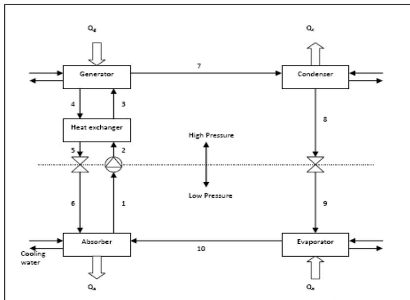
Figure 2: Schematic of a single effect liBr-water absorption system
