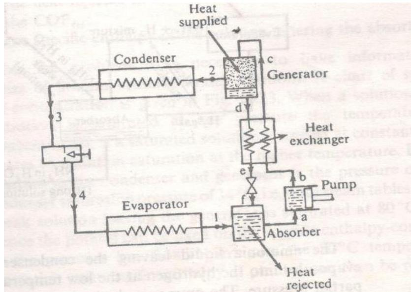
Figure 1: Diagrammatic arrangement of a vapour-absorption system
